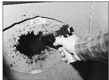
Step 16: Function test the gun. Here, Aronstein is shooting into a bullet trap with an angled backstop.
