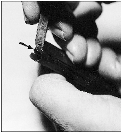
Step 11: Adjust the front of the rear lips of the magazine as needed. Keep the lips parallel.
